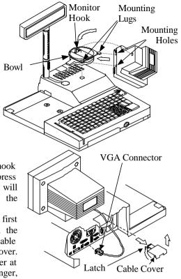
then raise and rotate the monitor forward till the CRT front is facing downward.
